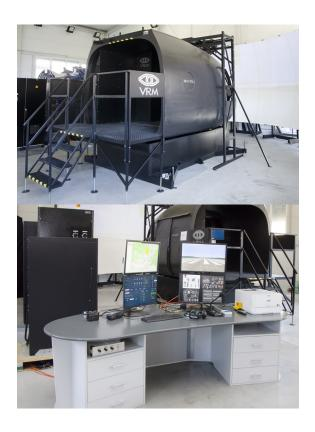
Control Loading System (CLS) and vibrating platform, provide accurate cues for the realistic training experience. Control forces and displacement characteristics correspond to that of the actual helicopter.
